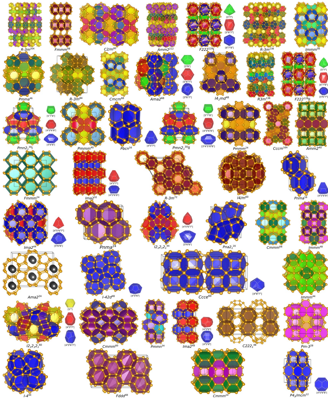
Figure 1: Polyhedral structure of the cages in low-density allotropes of silicon.
